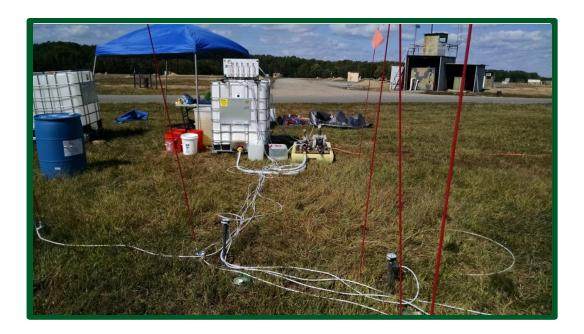
Passive Biobarrier for Treating Co-Mingled Perchlorate and RDX in Groundwater at an Active Range
