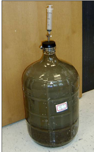
Figure 3-11. Macrocosm in 5-Gallon Carboy
