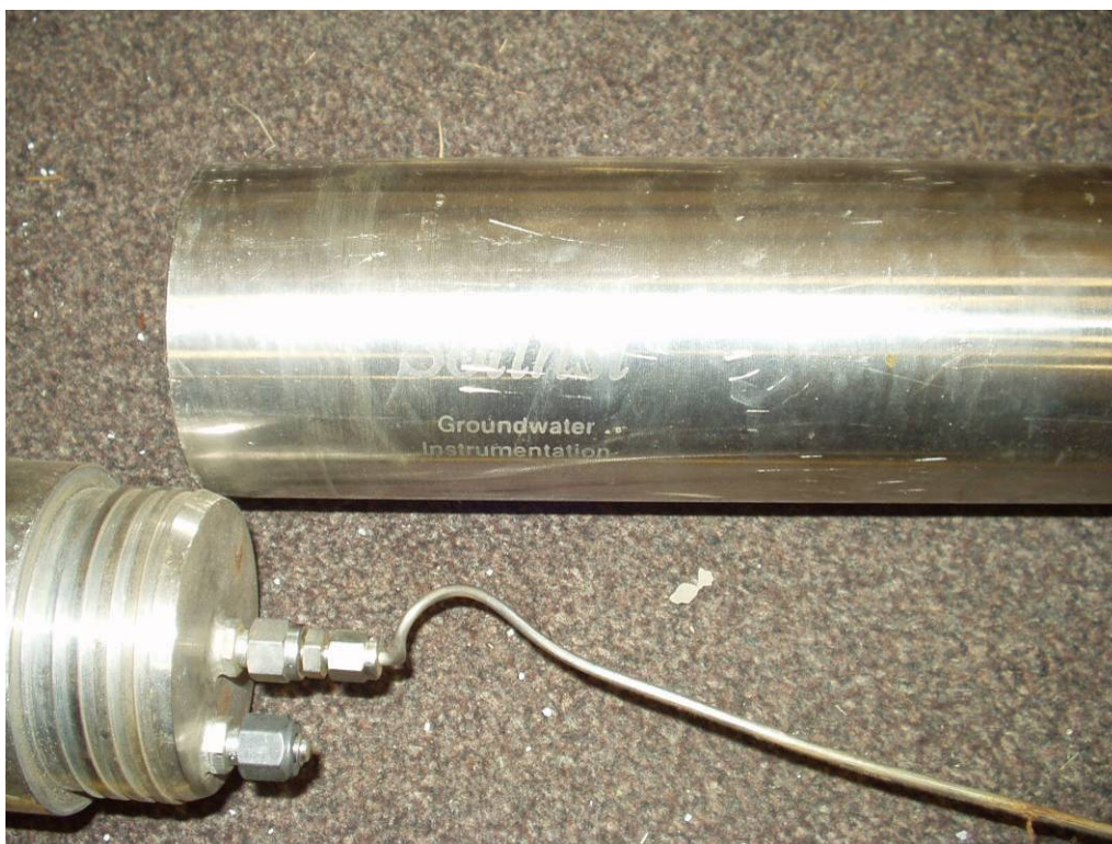
Figure 3-10. Stainless Steel Solinst ® In Situ Column Showing Sampling Port Attachment
