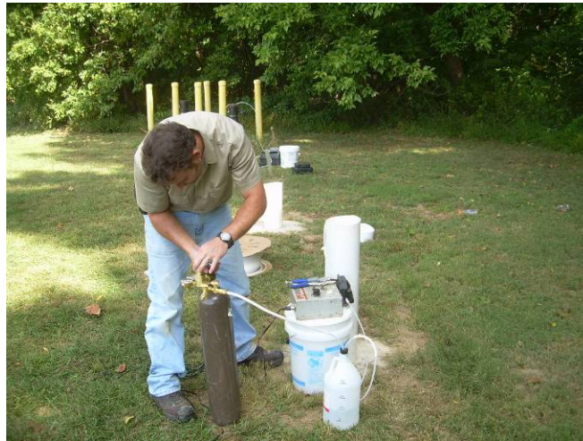
Figure 6-12. Amending In Situ Column ISC-A near GM-22S/M
