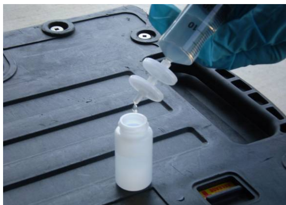
Figure 3-8. Field Preservation of Aqueous Perchlorate Sample by Filtration through a Filter Stack
