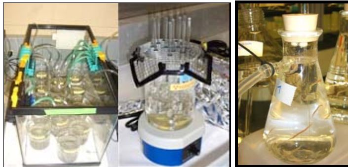
Figure 6. Picture of polychaete exposure setup to measure PCB uptake rates from sediment (left) and aqueous exposure studies with clams (middle) and polychaetes (right).
