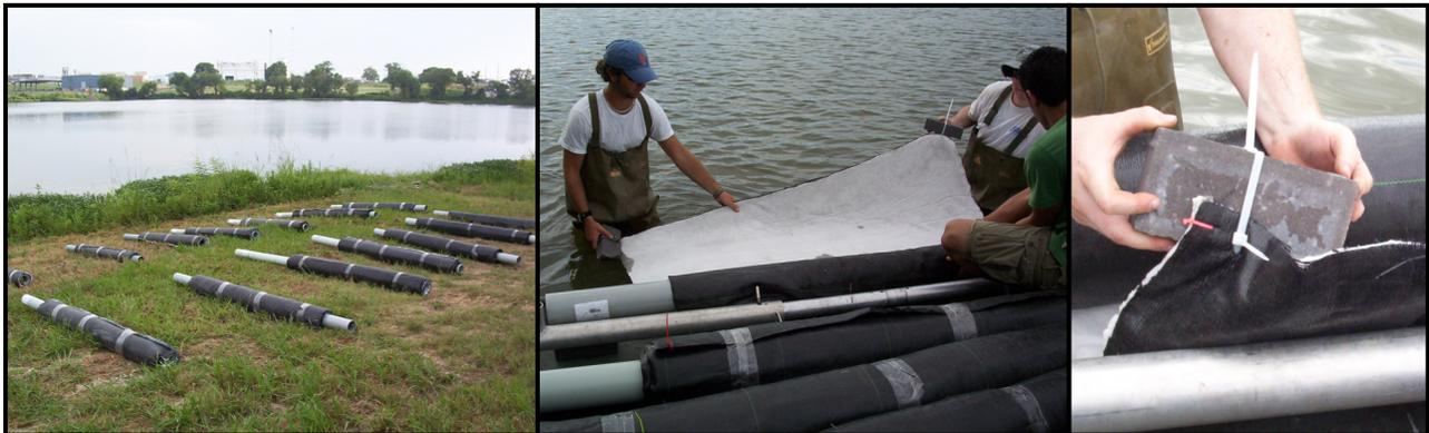
**Figure 6.3-2.** Small-scale geotextile test mat deployment.
