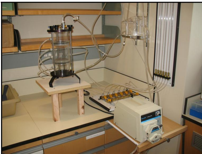
**Figure 6.3-4.** Geotextile permeability column experimental setup.
