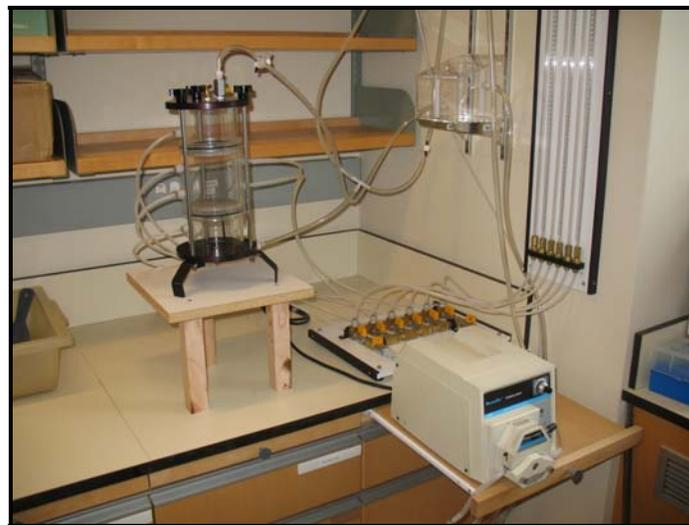
**Figure 6.3-1.** Permeability column test setup.
