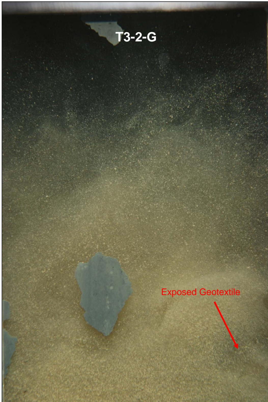
**Figure D-7.** Sediment profile image of prototype mat system area T3 (double mat) taken on top of geotextile.
