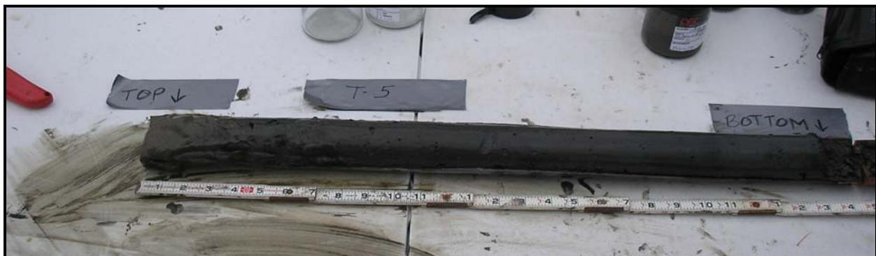
**Figure I-6.** Sediment core collected at control area T5 (no treatment).
