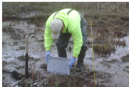
Figure 2-2 In situ Pore Water Sampler Courtesy EA Engineering, Science, and Technology, Inc.
