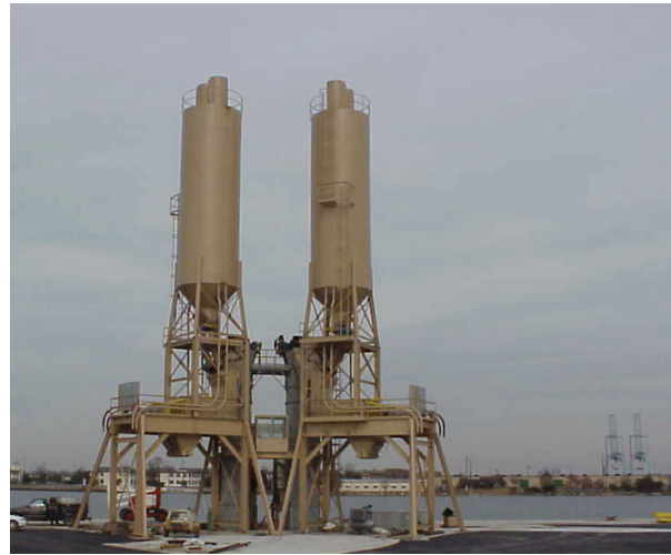
Gravity feed dual pugmill system
