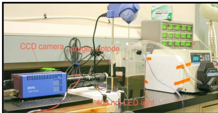
**Figure 4-8.** Oxygen optode experimental setup.
