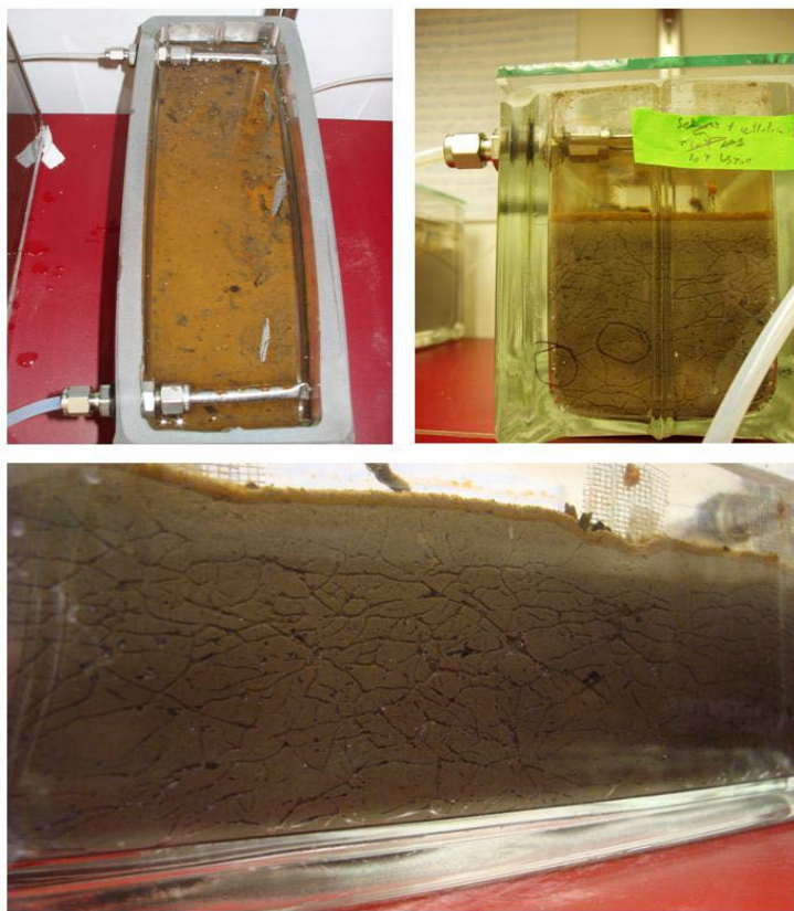
Figure 13. Mesocosm Showing Development of Distinct Oxidic and Anoxic Zones (all treatments) and Bioturbation Due to Active Burrowing by Benthic Organisms (Treatments 5 & 6).
