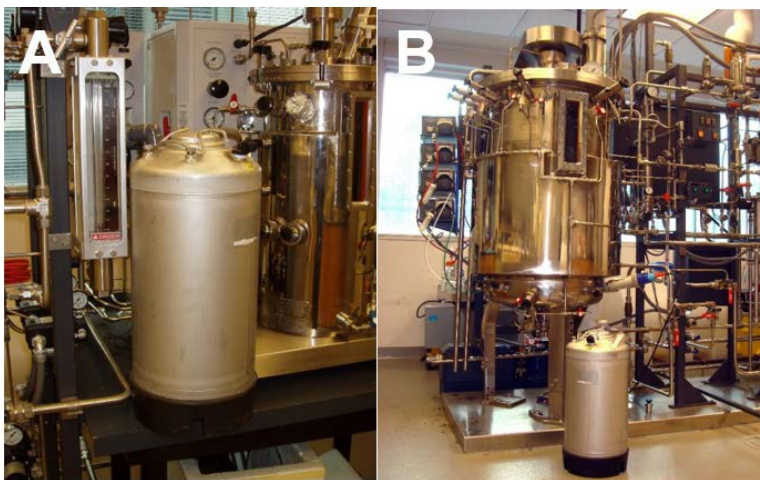
Figure 31. BioFlo Bioreactor (20 L) and Pilot-scale Fermentor (250-liter) at IMET-UMBC for Scale Up of Microorganisms.
