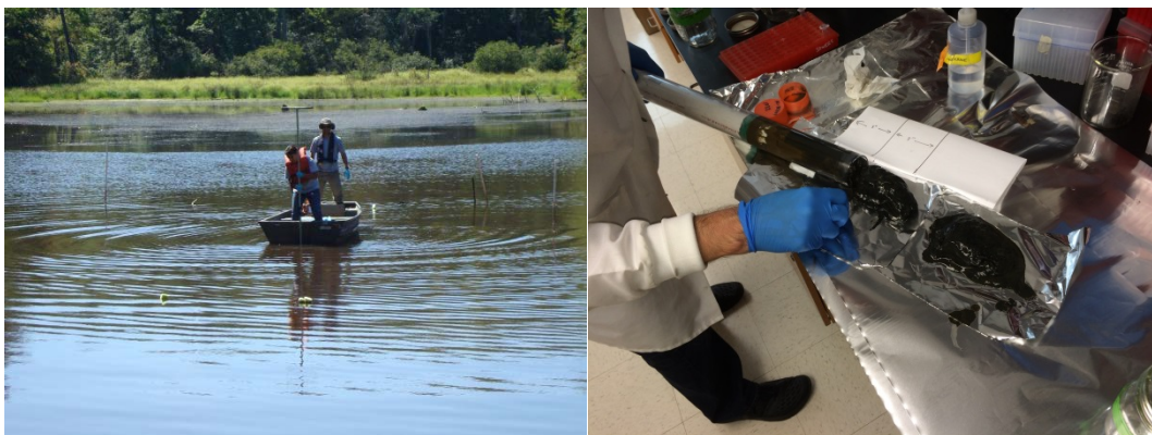
Figure 37. Sediment Sampling with 5 cm Polycarbonate Lined Core Sampler (A); Extrusion and Subsampling of 7.5 cm Subcores Section in the Lab (B).
