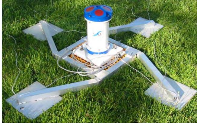
**Figure 3-7. Up-looking Acoustic Doppler Current Profiler (ADCP) (Teledyne RD Instruments 1200 kHz Workhorse Sentinel ADCP [Poway, CA]) on Bottom-Mount Platform for Measuring TSS.**
