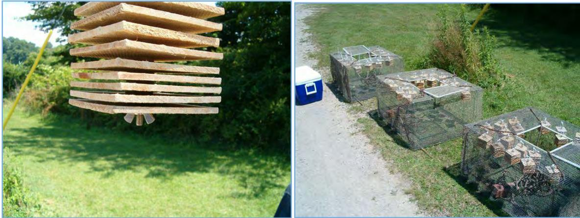
**Figure 2-9. Macrobenthos Samplers Used at Ashtabula River (Left –H-D artificial substrate plate sampler; Right – Samplers hanging in fish cages during deployment).**
