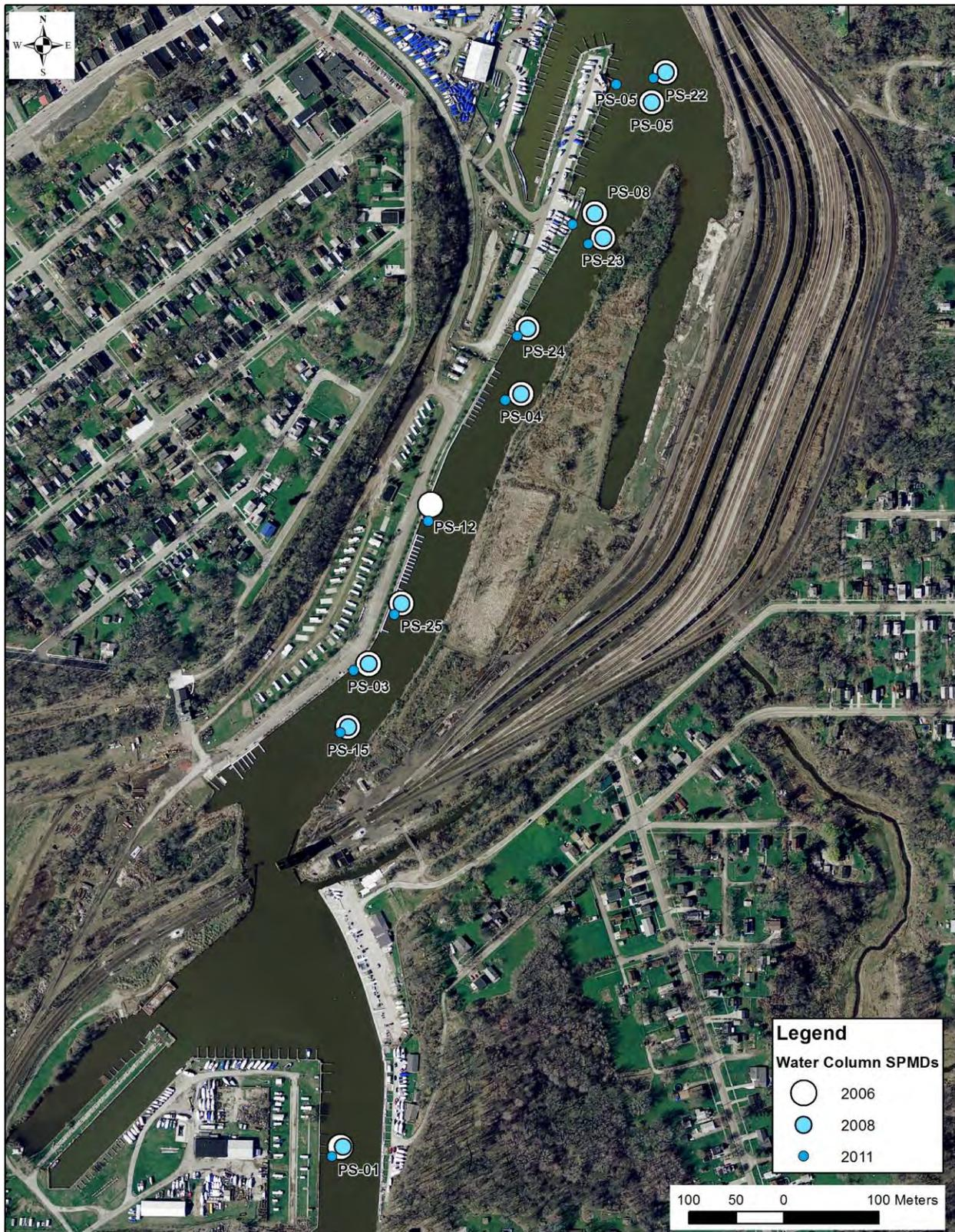
Figure 2-5. Water Column SPMD Deployment Locations.
