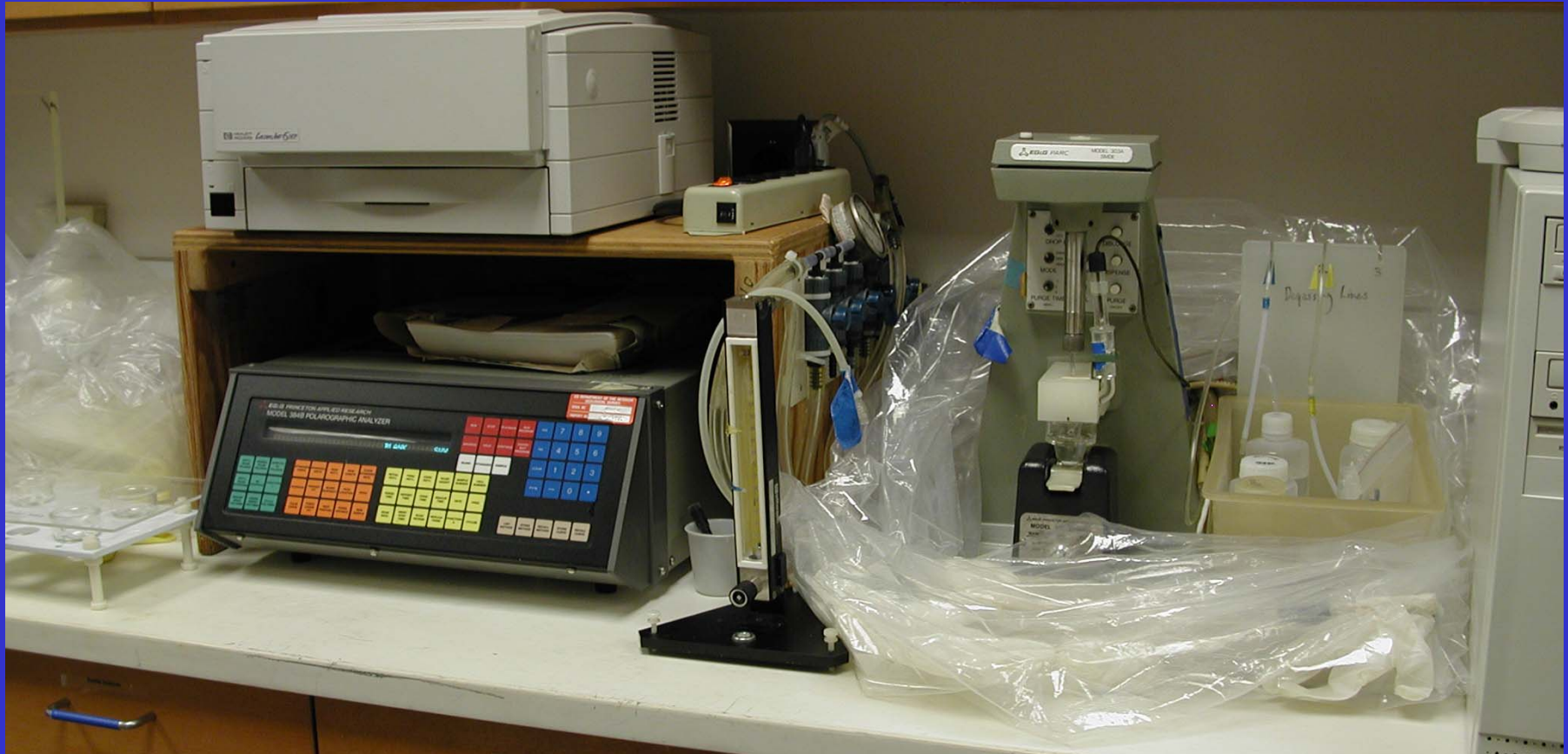
Fig. 17. Photograph showing polarographic equipment used for dissolved-sulfide analyses by square-wave voltammetry.
