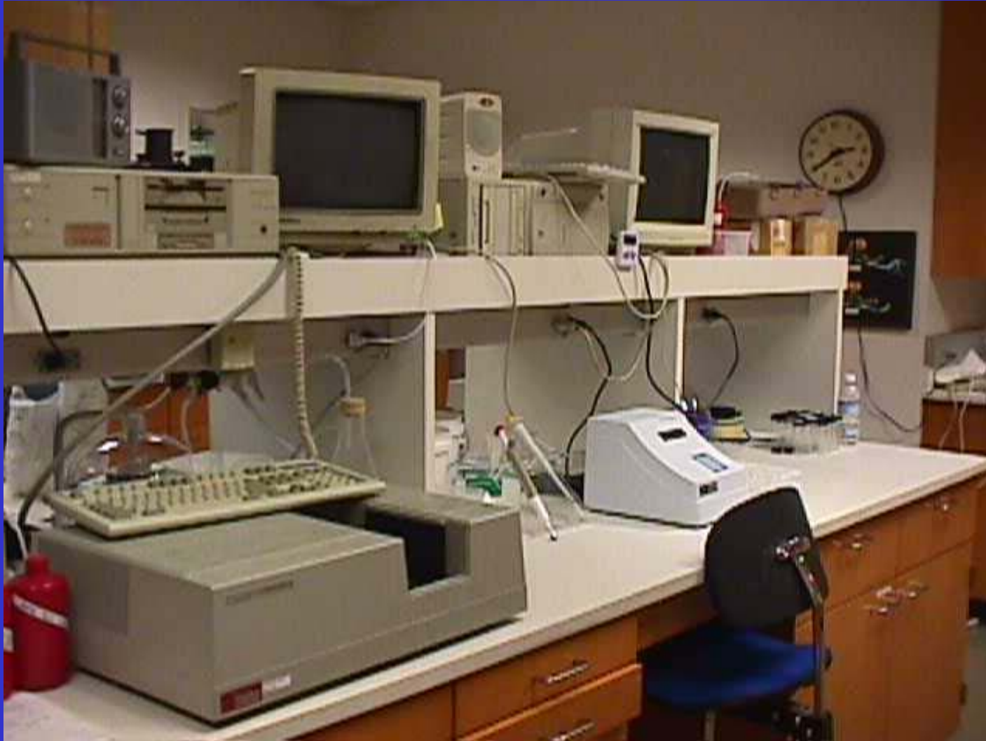
Fig. 13. Photograph showing spectrophotometric equipment used for benthic-chlorophyll analyses.
