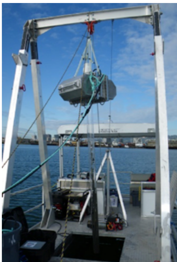
Figure 7. Vibracorer Deployed from Sampling Vessel (Courtesy of Battelle)
