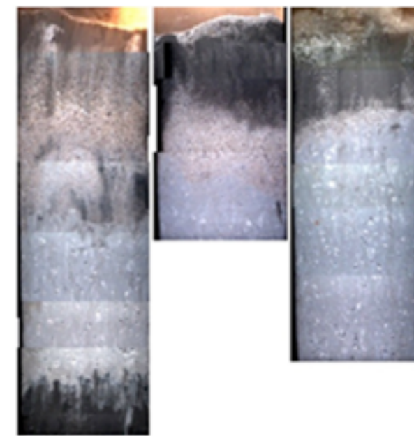
Figure 8. Vertical SPI Profiles Showing Variations in Material Type with Depth (Courtesy of Battelle)
