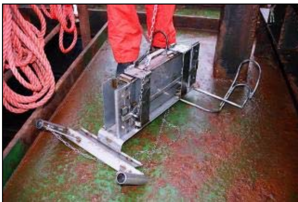
Figure 7.2. Overflow sampler (capacity 4 litres) used during the Rotterdam TASS protocol trial.
