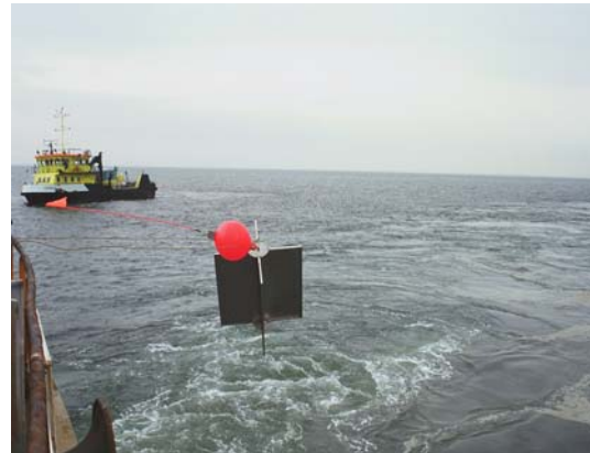
Figure 6.1b. A drogue being deployed from the stern of a trailer dredger.
