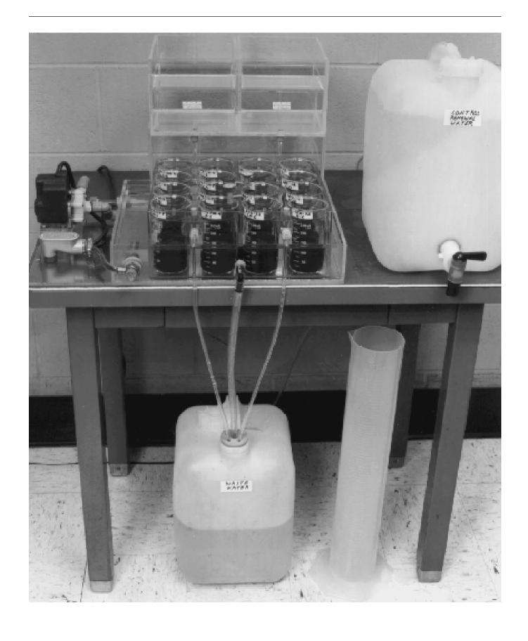
Figure A.1 Portable table top STIR system described in Benoit et al. (1993).
