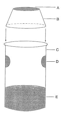
Figure C.1. Emergence trap used in the life-cycle *Chironomus* tentans sediment test. A: the nylon screen; B: the inverted plastic cups; C: the 300-mL lipless exposure beaker; D: the water exchange screen ports; E: test sediment.
