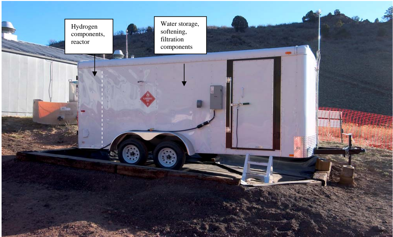
FIGURE 6 Photograph of Treatment Trailer (May 2006)
