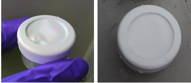
**Figure 6. Peeper with Membrane Damage (Left) and Peeper with No Damage (right).**
