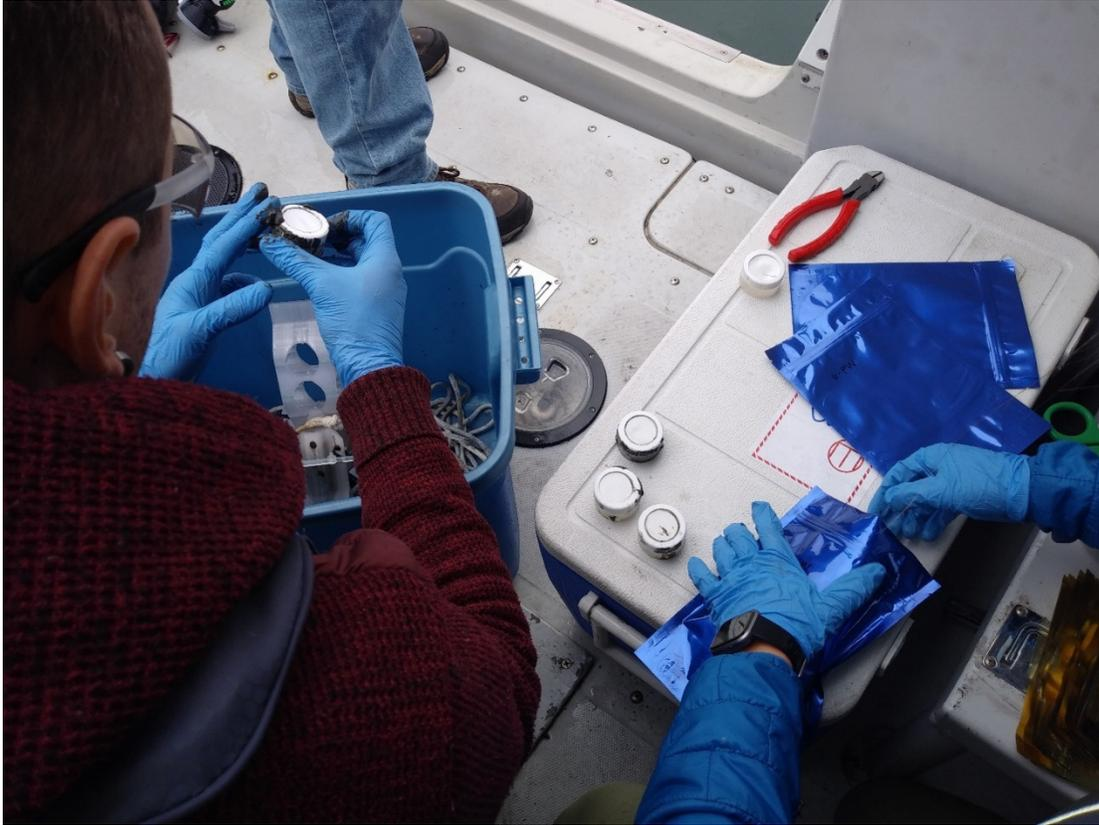
**Figure 11. Peeper and DGT Storing After Retrieval.**
