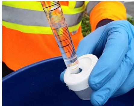
8. Dispense at least 5 mL from the peeper in the sample container for the bromine analysis (if bromine is being used as a tracer).
