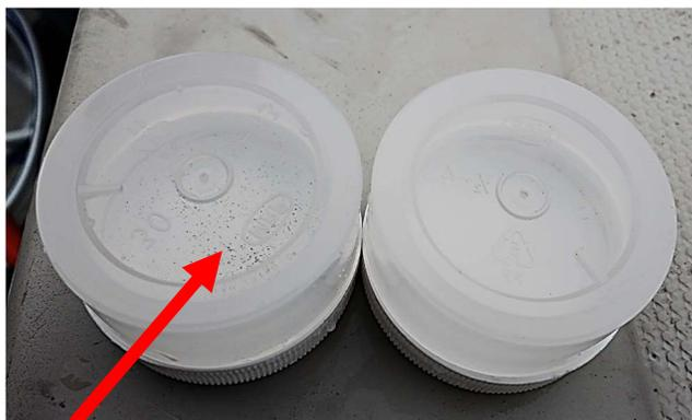
**Sediment grains** that have entered the peeper; they are observable by swirling the water and turning the peeper upside down
