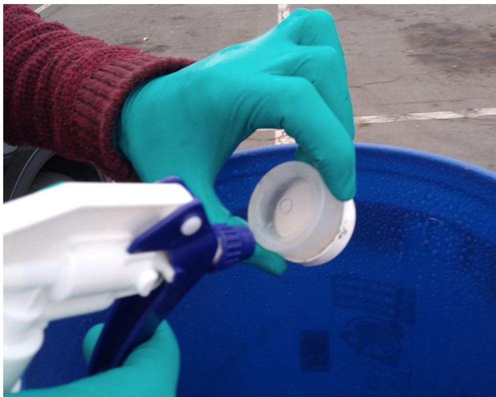
**Figure 13. Washing Peepers to Remove Sediments from the Membrane.**
