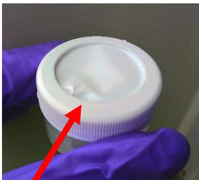
A **wrinkle** in the peeper membrane due to damage or mishandling; do not use the peeper for field deployment, although it can be used as a Trip Blank if needed
