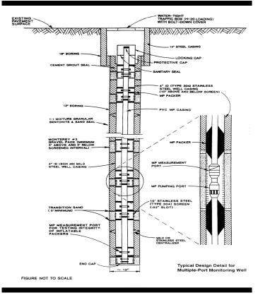
The following figure shows the typical design detail for a Westbay System multiport monitoring well.
