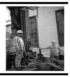
The Simulprobe<sup>TM</sup> provides continuous sampling of soil gas in the vadose zone. When the probe is pushed through the vadose zone, soil gas is extracted under the vacuum and measured continuously in an organic vapor analyzer located above ground surface. If desired, a syringe can be inserted and a sample of soil gas can be extracted and analyzed by gas chromatography (GC) at any time.
