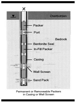
installed and maximizing the number of groundwater zones sampled. The purge volumes necessary for groundwater sampling using the Waterloo System are likely to be smaller than those from conventional nested monitoring wells.
