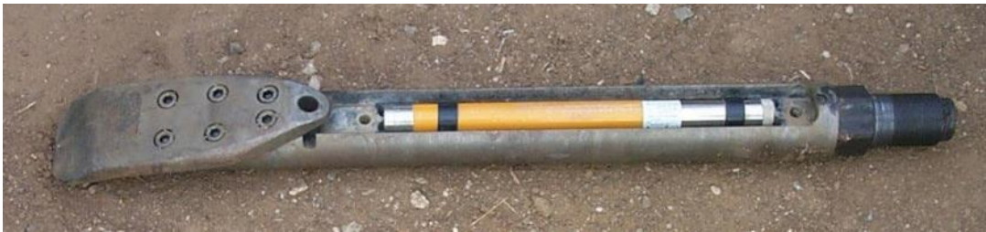
Exhibit A-9. Typical Drillhead (With Cavity Open)
