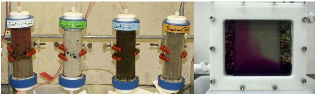
**Figure 2.8. 1-D Column Tests (left), and RemOx SR Mini-cylinder 2-D Tank Experiments (right).**
