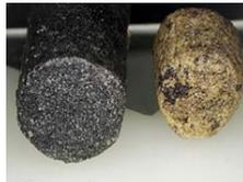
**Figure 2.5. New (left) and Spent (right) Permanganate Cylinders.**
