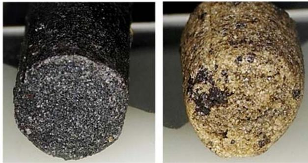
**Figure 2.** Photos of slow release permanganate cylinders. Left: Unused cylinder; Right: Used cylinder showing wax skeleton.
