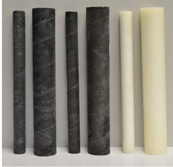
**Figure 2.6. RemOx SR (left), RemOx SR+ (center), and Persulfate SR (right) Cylinders Shown in 1.5- and 2.5-inch Diameters**
