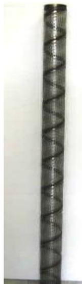
**Figure 2.14. Stainless-steel Mesh Cylinder Holder.**
