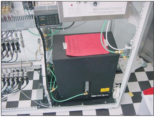
B-23. Oxygen Generator Pressure Swing Adsorption System
