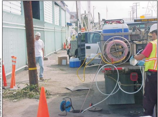
B-27. Groundwater Sampling at Monitoring Well MW-20
