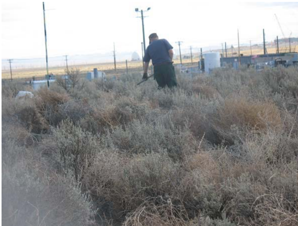
Figure M.6. Redistribution of imported tumbleweed across the barrier to achieve different fuel loads for the controlled burn. Captain Jerry Keeling of the Hanford Fire Patrol is shown redistributing tumbleweed with a rake. (After Figure 2.11 of Ward et al. 2009a).
