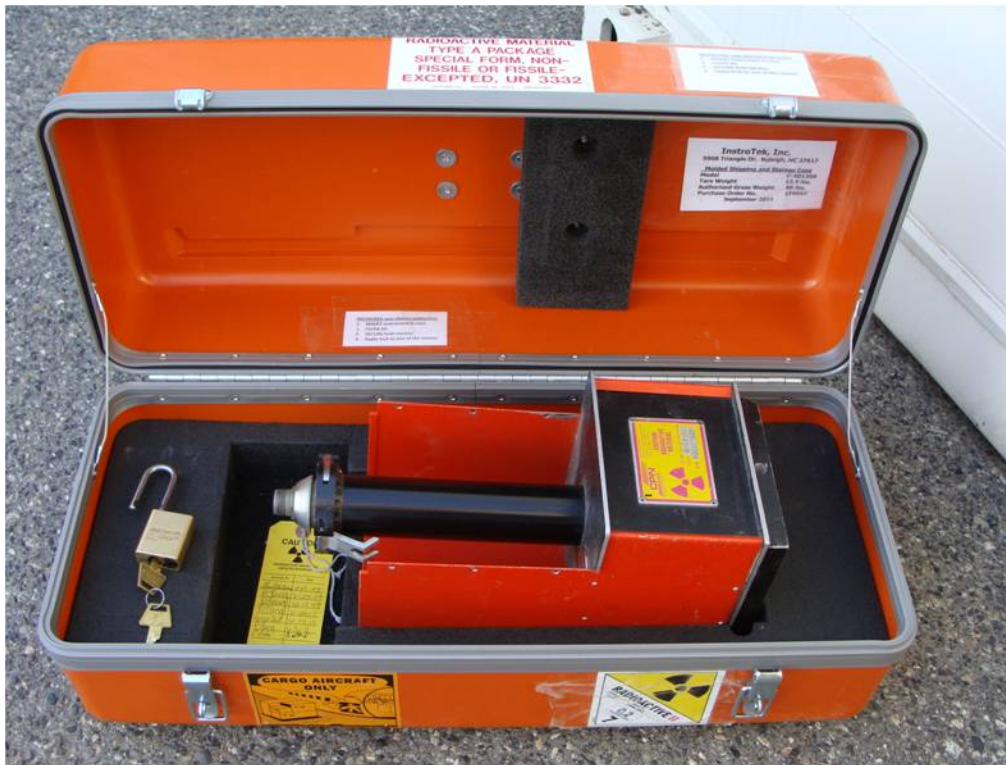
Figure C.3. A 503DR Hydroprobe for soil moisture logging.
