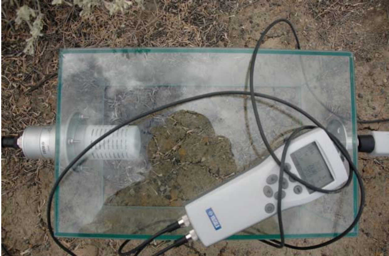
Figure K.1. Static Diffusion Chamber with Sensors and Readout Device
