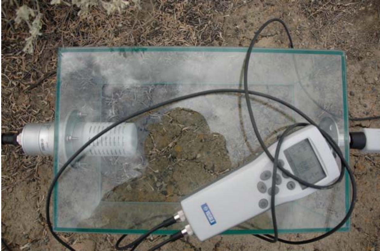
Figure C.14. Static diffusion chamber with sensors and readout device.
