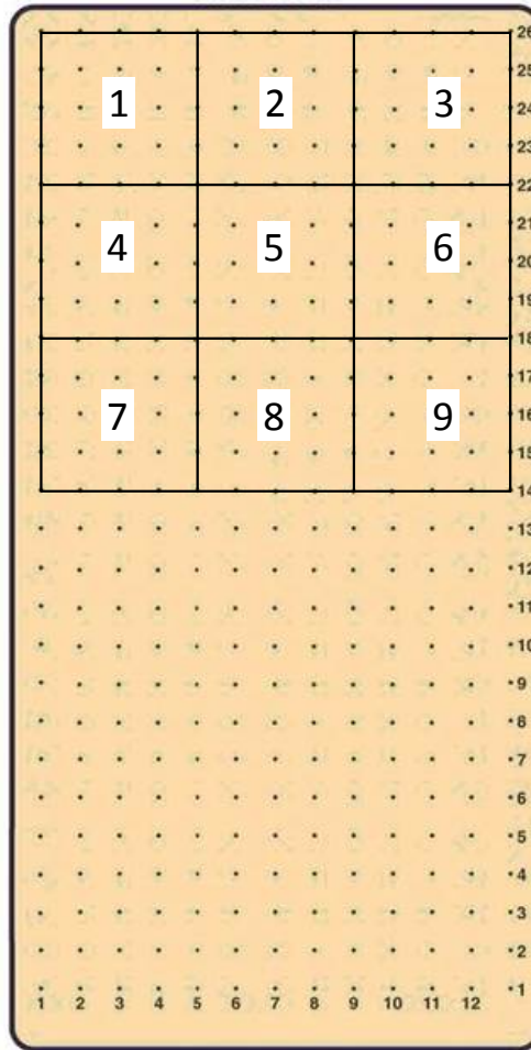
Figure M.1. Schematic plan view of the barrier's surface showing the 3 \times 3 m grid and the nine (1 through 9) 12 \times 12 m plots to be used for comparing effects of fuel loads on fire intensity.
