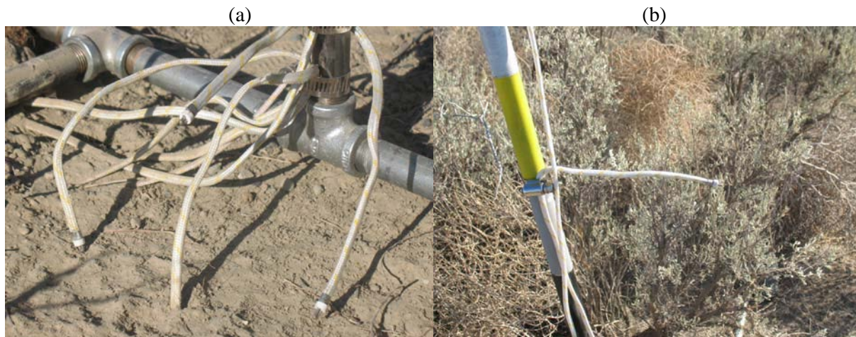
Figure M.3. Thermocouples for measuring soil and air temperature installed on flame height scaffold: (a) thermocouples were installed 1.5 cm deep, at the surface (0 cm), 1 cm, 10 cm, and 30 cm, and (b), aboveground thermocouples were installed at 100 cm and 200 cm (After Figure 2.8 of Ward et al. 2009a).
