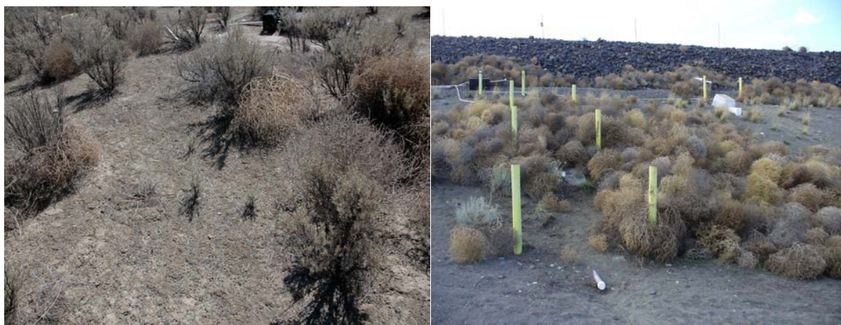
Figure M.4. Photographs of the PHB surface: (a) sparse vegetation on the surface suggesting need for increased fuel load to emulate realistic conditions. Some Salsola kali (tumbleweed) was already lodged among sagebrush plants, and (b) the riprap side slope of the barrier shows an accumulation of tumbleweed. Dead sagebrush and tumbleweed were imported to the barrier surface to increase the fuel load. (After Figure 2.9 of Ward et al. 2009a).
