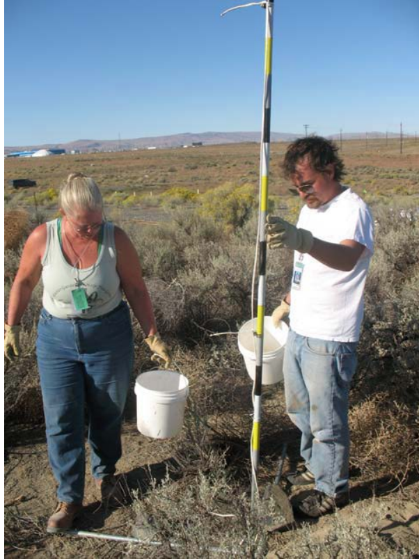
Figure M.2. Photograph of fire pole used to measure flame characteristics and to secure thermocouples (After Figure 2.7 of Ward et al. 2009a).
