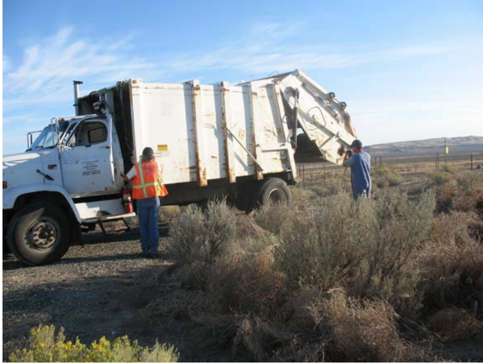
Figure M.5. Unloading of tumbleweed brought to the barrier to increase fuel load. Over 2 tonnes of tumbleweed was added to the surface. (After Figure 2.10 of Ward et al. 2009a)
