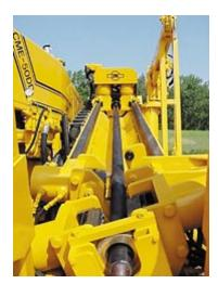
For remediation of contminant plumes, horizontal wells can offer significant advantages over vertical wells. Courtesy of Central Mine Equipment Co.
