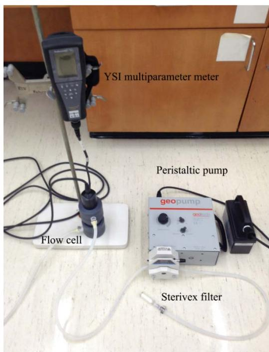
**Figure 1.** Set-up of our groundwater sampling equipment
