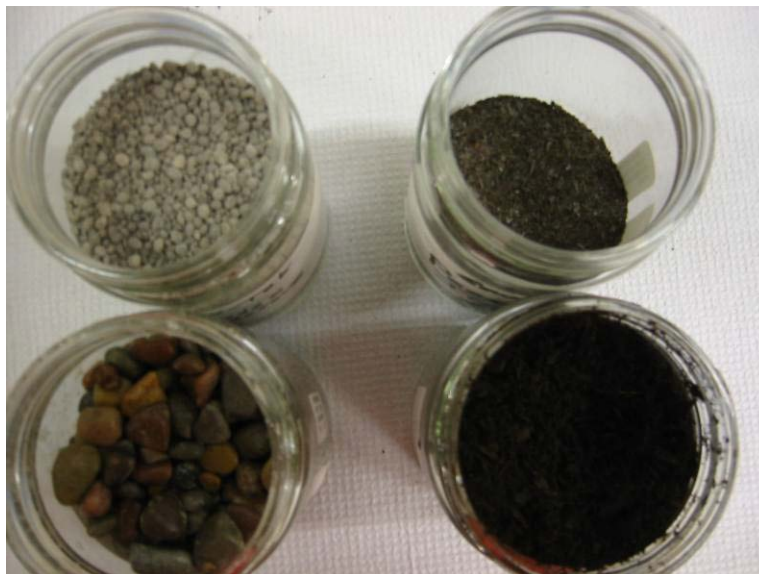
Figure 4-11. Components for a biowall-ZVI PRB bench test. Clockwise from top left: limestone, granular ZVI, leafy compost, gravel.
